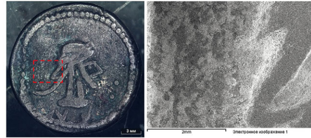
Fig. 45. The studied area (a), the electronic image (b) of the surface of Pharsanzes' stater No. 2136, and the total characteristic spectrum from the studied area of surface (c).
