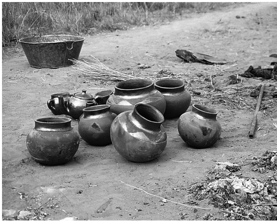
Fig. 13: Pots just after firing in an open fire. Traditional vessels (front) and imitations of European vessel types such as kettles (at the back). Note the elaborate use of graphite on the latter to imitate the luster on metal vessels.
