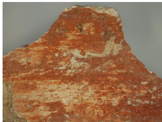
Fig. 4.: The most common red pigment is red ochre, i.e. red earth consisting of mixed iron oxides. The pigment layer is damaged, but the regular strokes can still be recognized. The plaster is white, compact and without sand. Magnification 50x. (Photo by authors)
