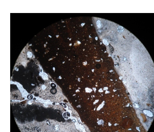
Fig.4 S-2 Large fragment of brick with quartz grains inside
