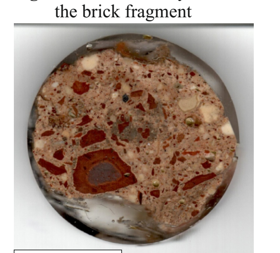
Fig.11 S-13 Dark border on some fragments of brick
